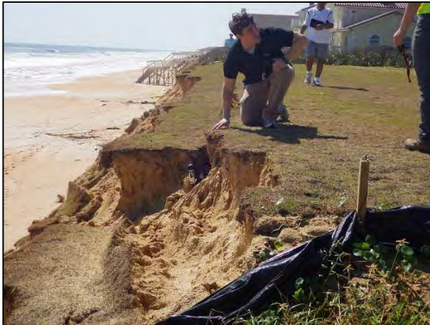
c) Close up of blocky nature of failed dune crest (Latitude 29°32'36.74"N / Longitude 81°9'29.95"W).
